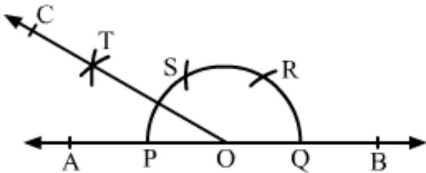
With a convenient radius and centre at O, draw an arc, which cuts the line AB at P and Q.
