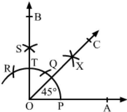
To construct an angle of  $45^\circ$ , construct an angle of  $90^\circ$  and bisect it.
