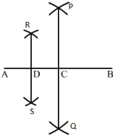
(i) With A as centre and radius more than half of AB, draw arcs on both sides of AB. (ii) With the same radius and B as centre, draw arcs cutting the arcs drawn in step (i) at P and Q.
