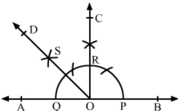
With a convenient radius and centre at O, draw an arc, which cuts AB at P and Q, respectively.
